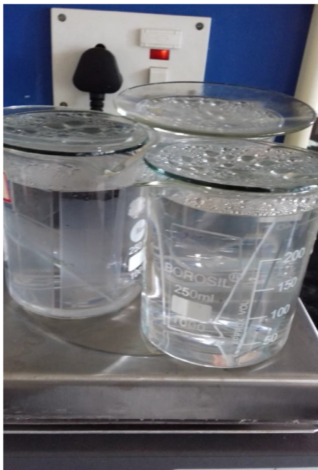
FIGURE 2 Experimental setup for the selective dissolution of PEO from PEO-PMMA polymer nanofibers [Color figure can be viewed at wileyonlinelibrary.com ]
