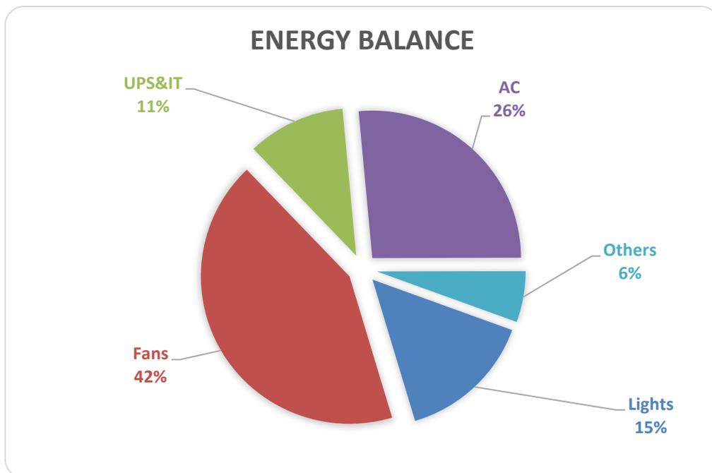
In this facility, the breakdown of energy consumption reveals that fans contribute to 42%, lighting utilizes 15%, UPS and IT uses 11%, miscellaneous uses make up 6%, and air conditioning systems account for the remaining 26% of the total energy consumption.
